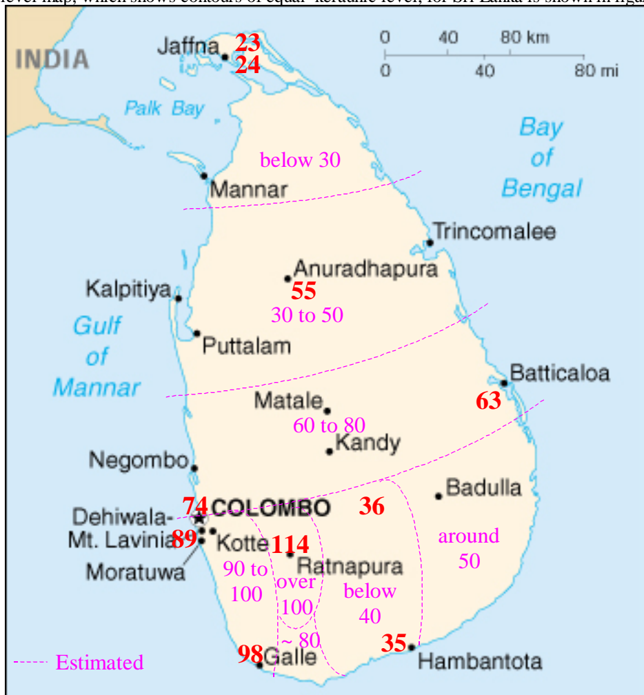
Figure 3.3 - Isokeraunic Level map of Sri Lanka
