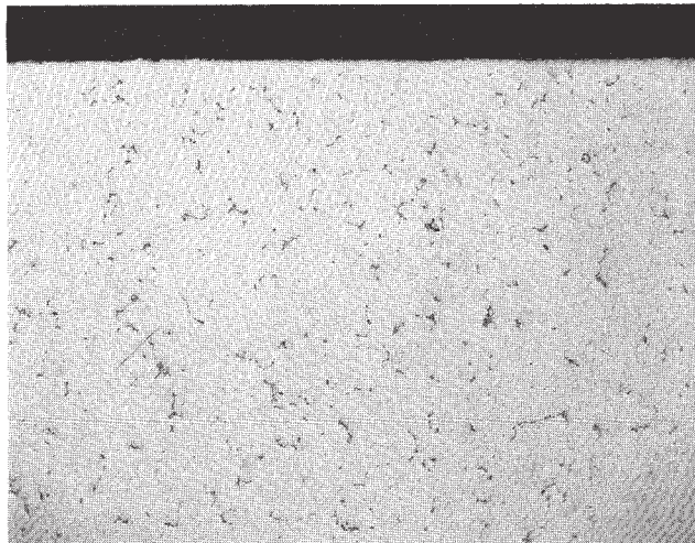
Fig. 1 The structures at the surface of several Hazelett-cast aluminum alloys. Magnif. 100x.
