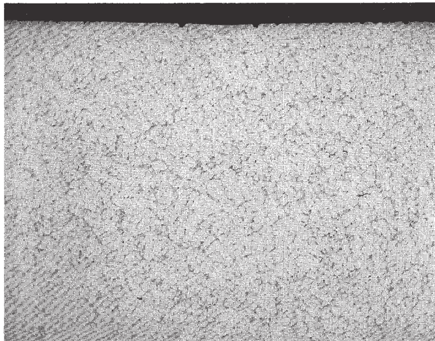
Fig. 1 The structures at the surface of the Hazelett-cast aluminum alloys.
