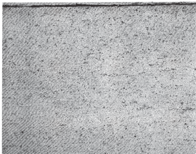
Fig. 5 Photomicrographs of alloy AA3004 showing progressive increase in structure homogeneity after various stages of processing.
