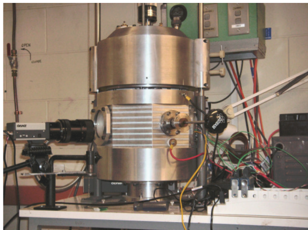
Figure 6. Chamber used for heat flow experimentation. The two sections of the chamber are visible, plus the external actuators, digital camera, and inlets and outlets for various services.
