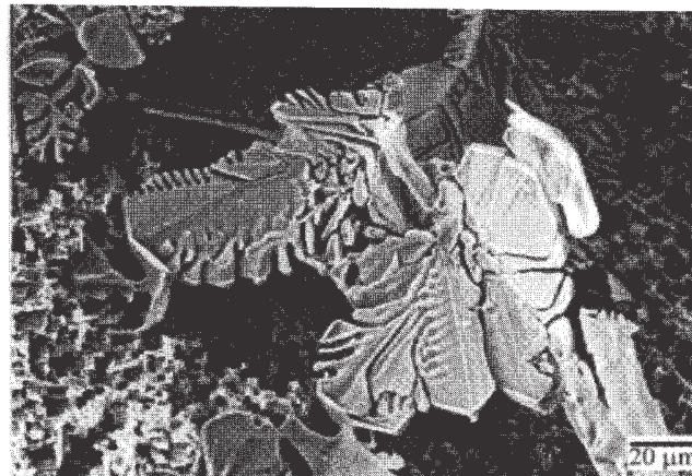
Figure 10: Three-dimensional view of \alpha\text{-AlFeSi} in the ingot structure (SEM, deep etched).
