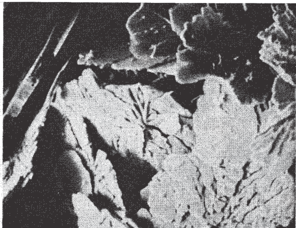
Figure 7. Scanning Electron Microscope Photomicrograph Showing Needle TiAl_3 Structure
