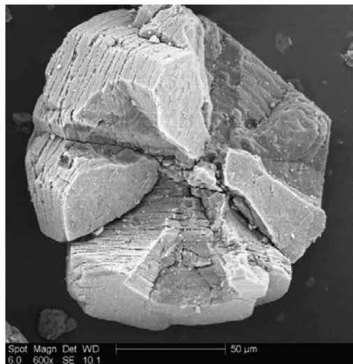
Figure 1. 600X magnification of a calcined alumina particle.
