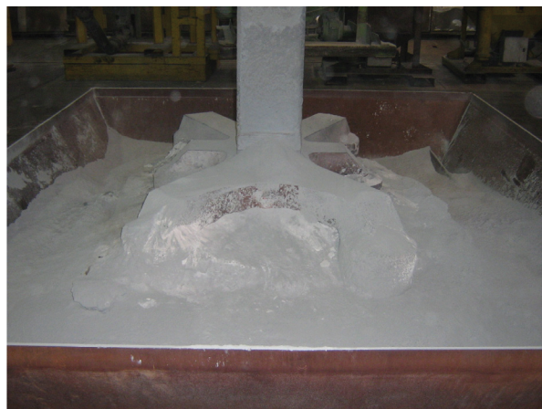
Figure 9 - Spent anode covered with cover mix
