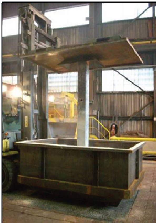
Figure 8 - Sealed anode box used for the proof of concept test
