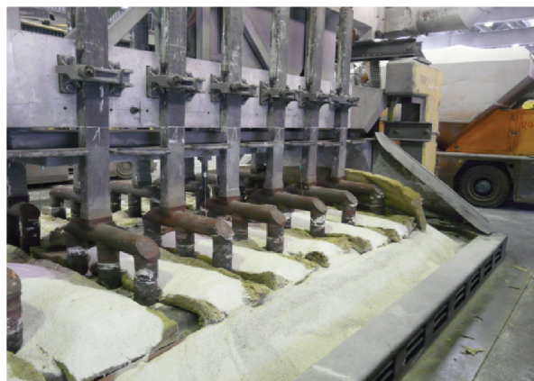
Figure 2: Test setup of cell in Potline 2
