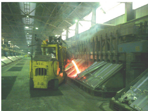
Figure 8: Liquid bath addition to cell 1035
