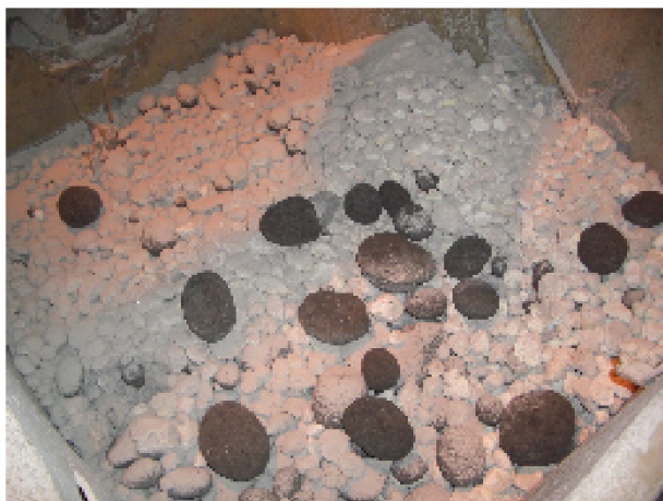
Figure 4: Material removed from mill during cleaning.
