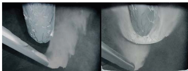
Figure 5 – 100% plugged recirculation point (left) and normally functioning alumina injectors (right). Fresh alumina at bottom.
