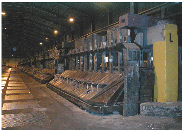
Figure 1. End-to-end point-fed prebake cells in the Sunndal III potline.
