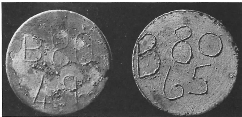
Fig. 4. Durability of RHM electrodes under cell conditions. Left: 2½ in. diam rod after 267 days of service. Right: unused rod.
