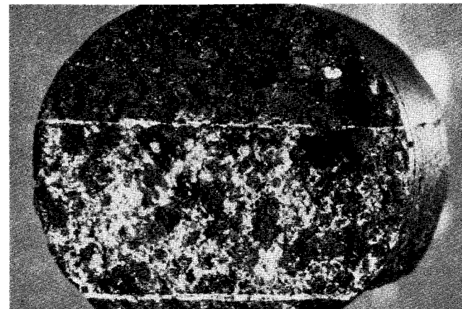
Fig. 1. Core sample from a failed prebaked cathode type cell shows prebaked block (upper and lower part) and seam (middle part). The "white" phase seen throughout the seam is mainly \text{Na}_3\text{AlF}_6 , \text{NaF} and yellow \text{Al}_4\text{C}_3 (4).
