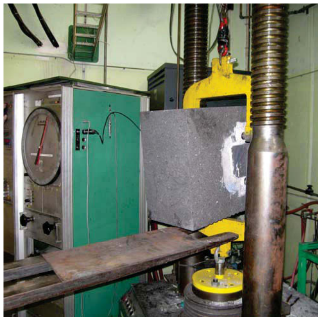
Figure 10. A cathode block section mounted in the test machine.
