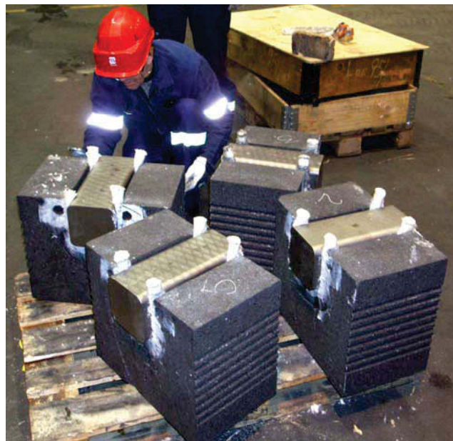
Figure 7. Bottom block sections made ready for preheating/cast iron pouring.
