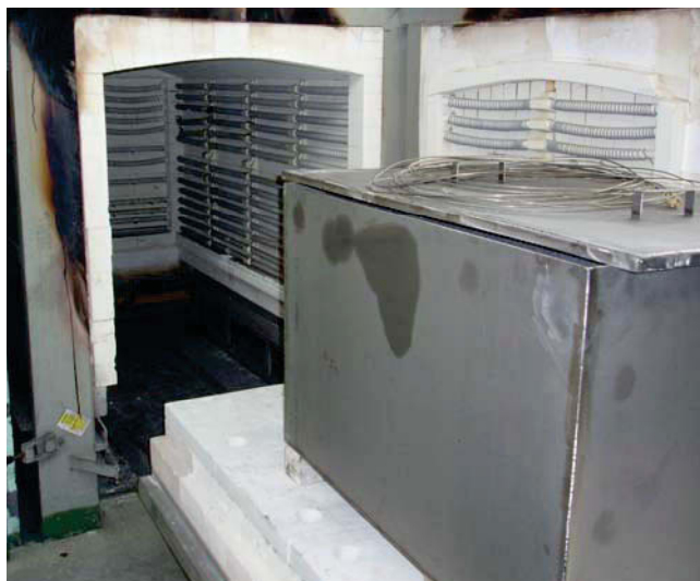
Figure 8. The steel box containing the rod sections were heat treated in a furnace to simulate the cathode preheating procedure.
