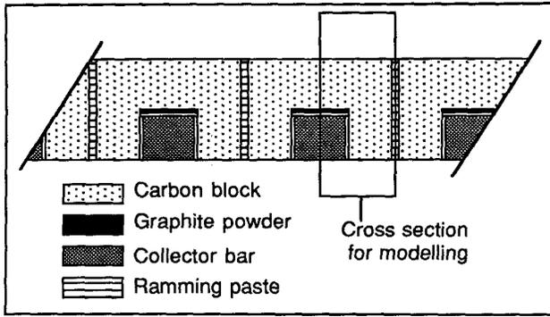
Figure 1. Cross section of part of the carbon bottom pane shows the selected part for modelling.
