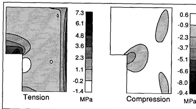
Figure 9. Stress fields in a block where the horizontal movement restrictions have been removed (Case 5).
