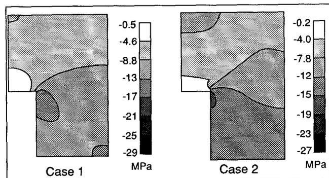
Figure 6. Compressive stresses in the bottom block without (Case 1) and with a 2.5 cm (Case 2) layer of graphite powder between the bar and the slot bottom.
