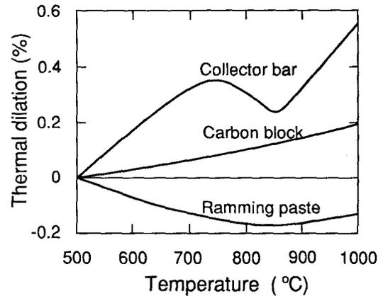
Figure 3. Thermal dilation of current collector bar, carbon block and ramming paste in the temperature range between paste baking ( $\approx 500^\circ\text{C}$ ) and cell operating temperature.
