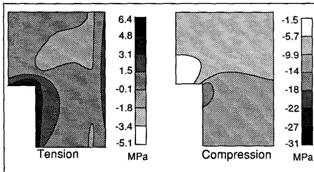
Figure 10. Stress fields caused by high friction between collector bar and carbon block (Case 6).
