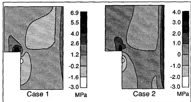
Figure 5. Tensile stresses in the bottom block without (Case 1) and with a 2.5 cm (Case 2) layer of graphite powder between the bar and the slot bottom.
