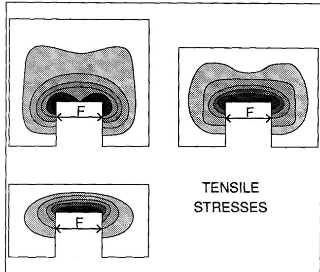
Figure 11. Shift in tensile stresses due to change in carbon block geometry. The darkest areas represent the highest stresses.
