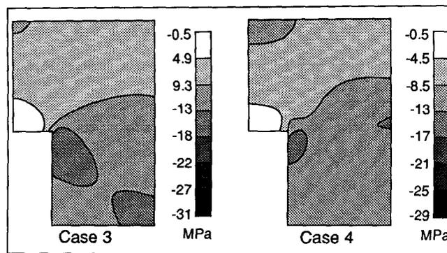
Figure 8. Compressive stresses with and without density gradient in the baked joint. Case 3: Uniform ramming paste density. Case 4: Uneven density in rammed joint.
