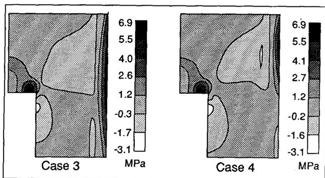
Figure 7. Tensile stresses with and without density gradient in the baked joint. Case 3: Uniform ramming paste density. Case 4: Uneven density in rammed joint.
