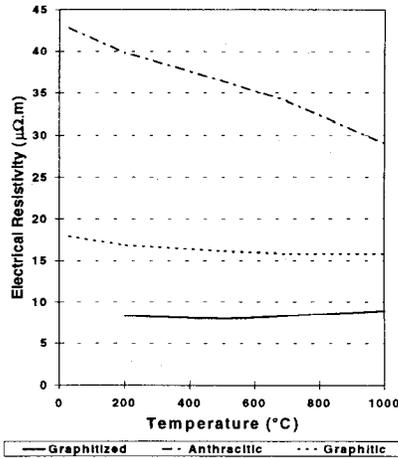
Figure 1: Electrical resistivity of different cathode blocks (along grain direction) [7]
