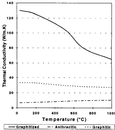
Figure 2: Thermal conductivity of different cathode blocks (along grain direction) [7]
