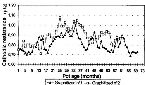
Figure 7 : pots with 2 different graphitized blocks (not boosted) - smelter B
