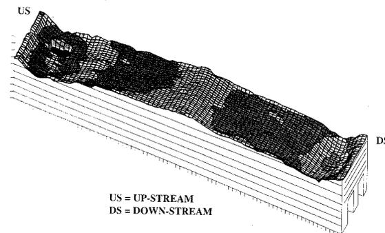
Figure 9 : Eroded graphitized block of a high intensity pot (61 months old) - smelter A.
