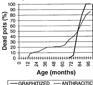
Figure 8 : pot life comparison between pots with anthracitic and graphitized blocks - smelter D
