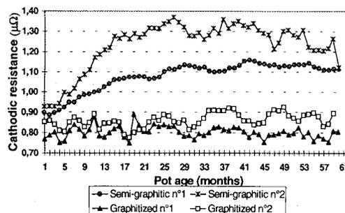
Figure 5: pots with semi-graphite blocks and graphitized blocks (boosted)- smelter A
