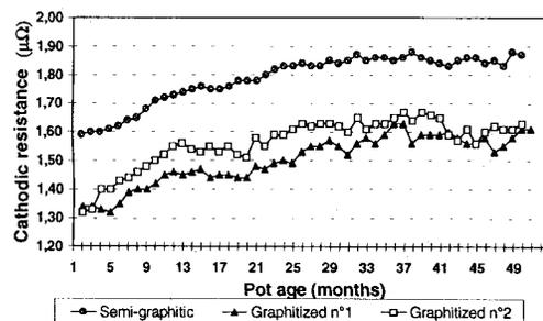
Figure 6: pots with semi-graphitic block and graphitized blocks (boosted) - smelter C
