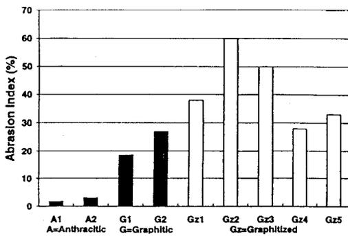
Figure 3: Abrasion resistance for different cathode blocks - grinding method
