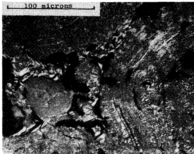
23. CO 2 -Oxidation Failure on Binder Side of Bond Between Fluid Coke and Coal-tar Pitch Coke
