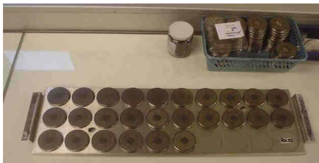
Figure 3. Tray with samples for x-ray diffraction analysis for L_c .
