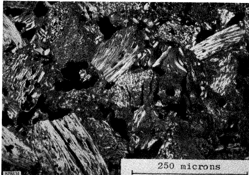
Figure 9 Microstructure of Baked, Well-Mixed, Compacted Anode Paste
