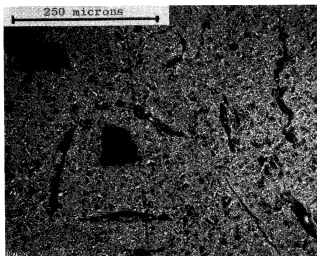
Figure 4 Disordered Filler Coke Structure
