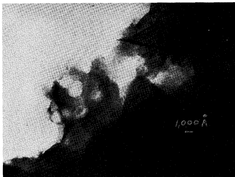
12. Empty Cavities in Coal-Tar Pitch Binder Coke Formerly Occupied by QI Particles which Fell Out Due to Poor Bonding
