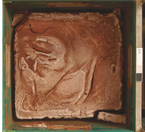
Figure 6(d). NaCl replaced (100%) residue surface at 16 weeks. NaCl efflorescence was strongly adherent and no friable red dust formed.
