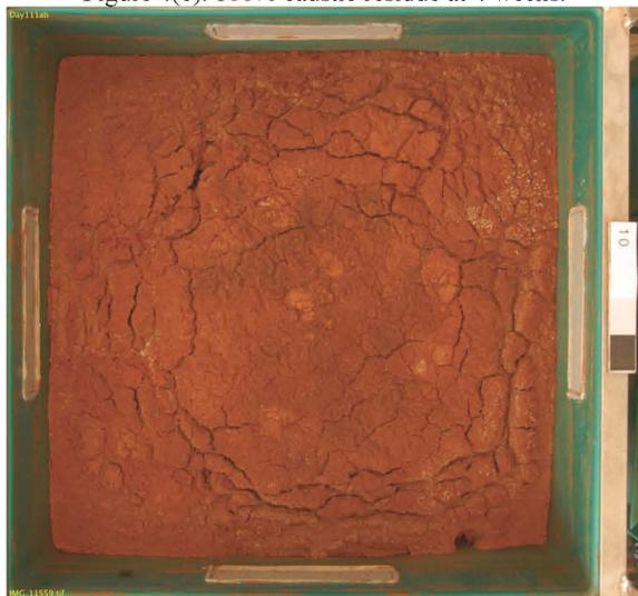
Figure 4(d). 100% caustic residue at 16 weeks with white dust overlayer removed revealing friable red dust.
