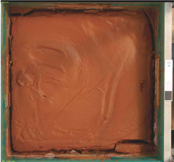
Figure 6(b). NaCl replaced (100%) residue surface at 2 weeks.
