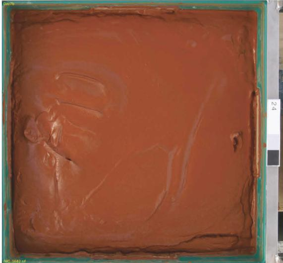
Figure 6(a). NaCl replaced (100%) residue surface at 1 week.
