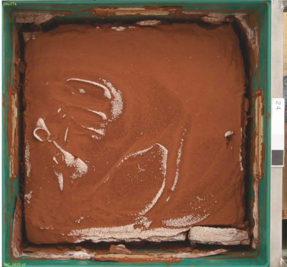
Figure 6(c). NaCl replaced (100%) residue surface at 4 weeks.
