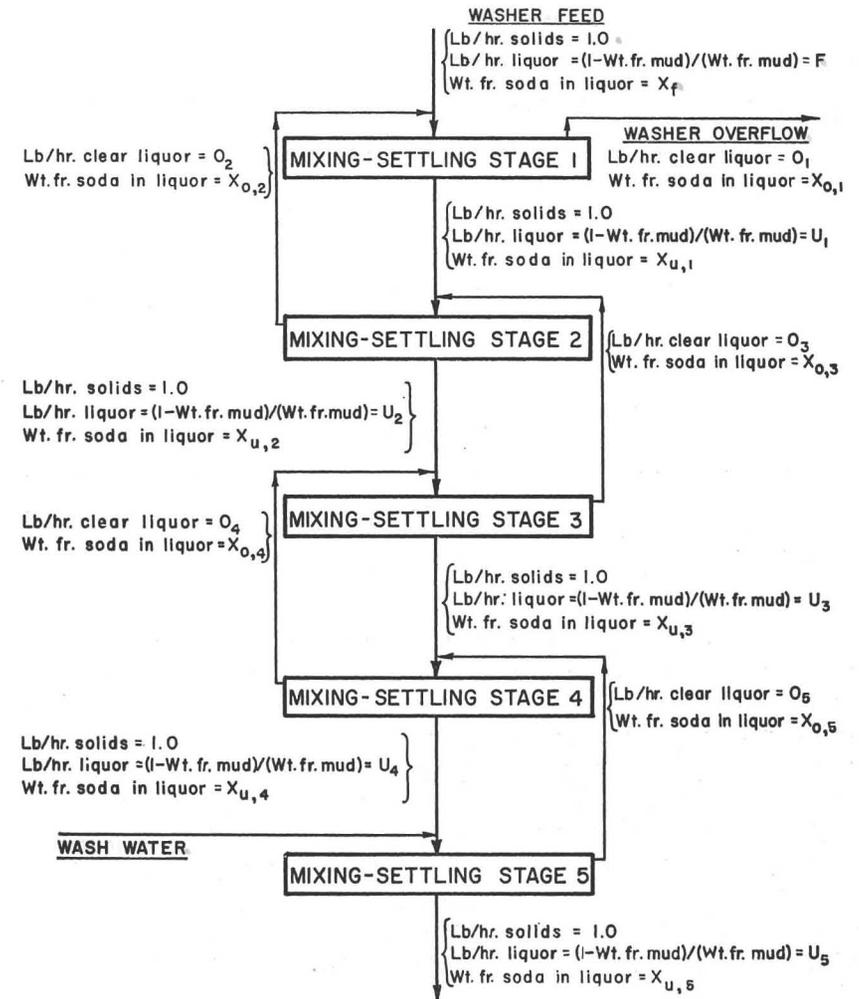
Fig. 1. Five-stage countercurrent washer.
