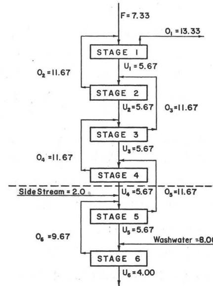
Fig. 2. Six-stage countercurrent washer with side stream.
