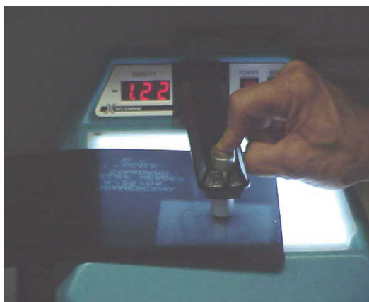
Film Density Measurement for 10" dia. x .500" thk. Pipe with 1" Thick Scale
