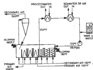
Fig. 8 Fluidized bed cooler with 3-stage counter-current water cooling.
