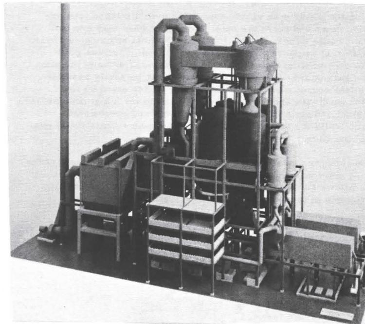
Fig. 7 Lay-out model of two parallel 1100 sh. t. p. d.  $Al_2O_3$  calcining units.
