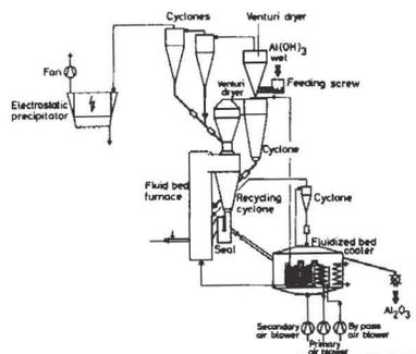
Fig. 2 Flowsheet of the first 560 sh. t. p. d. fluid bed calcining plant.
