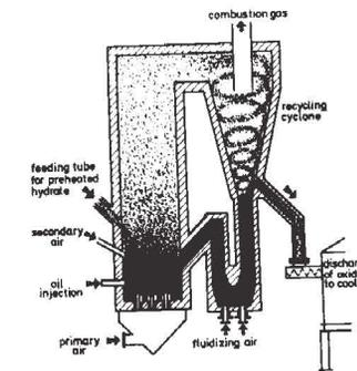
Fig. 1 Principle of the circulating fluid bed calciner
