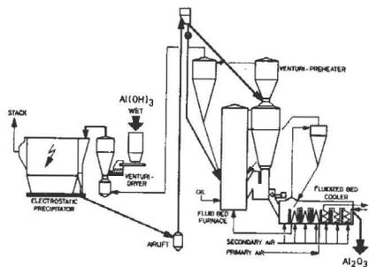
Fig. 6 Principal flowsheet of circulating fluid bed calciners with spread out arrangement.
