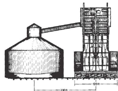
Fig. 3 Tower arrangement of 4 circulating fluid bed calcining units with a total capacity of 2900 sh. t. p. d.  $Al_2O_3$ .
