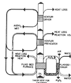
Fig. 9 Heat flow diagram for a 900 sh. t. p. d.  $Al_2O_3$  calcining plant (related to 1 lb. of produced  $Al_2O_3$ ).
