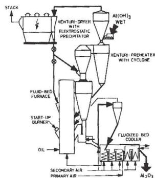
Fig. 4 Flowsheet of simplified circulating fluid bed calcining plant.
