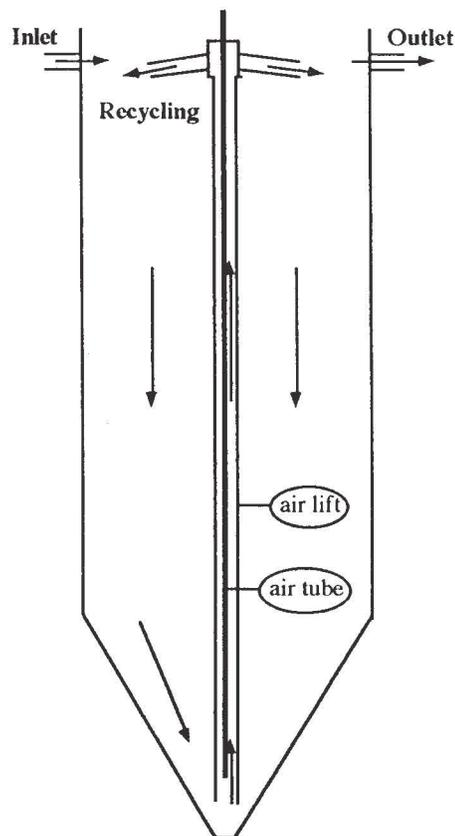
Figure 1 : design of original precipitator
