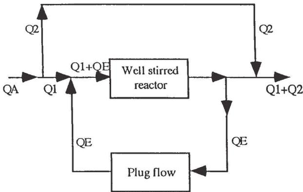
Fig. 2 Flow diagram of precipitator of fig. 1.
