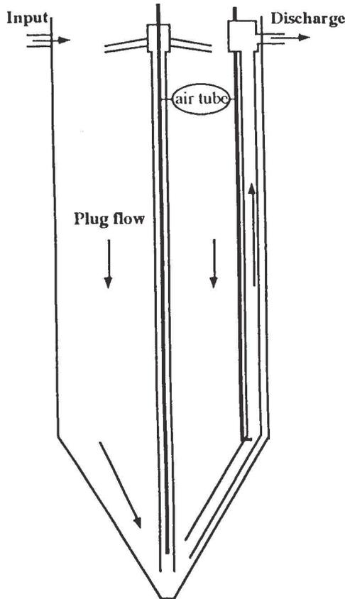
Figure 4 : bottom discharge precipitator
