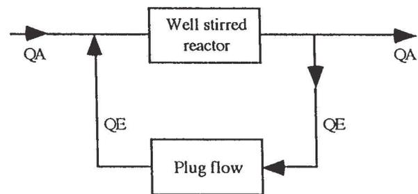
Figure 3 : flow diagram of tank with no direct short-circuit
