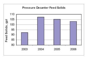
rate. The trend below shows the increase in the mono-hydrate content from 2002 to 2005 of the bauxite used at Gramercy. This increase in mono-hydrate content causes an increase in the feed solids to the decanters. The decanters were designed for a feed solids of 70 g/L. Today, the feed solids range from 70 g/L to 125 g/L.
