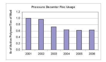
Flocculant has not been the only focus for decanter improvements. Key changes have been directed at improving underflow pumping capabilities to accommodate mud loads due to increasing mono-hydrate content of Jamaican bauxite.
