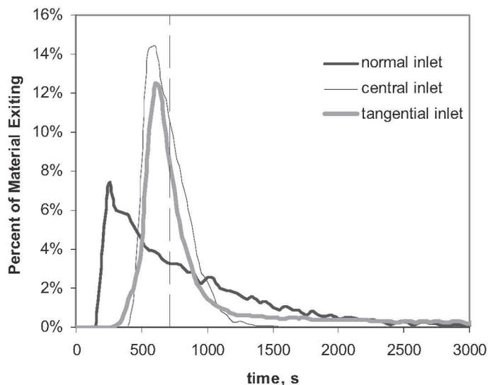
Figure 6: Single digester RTD. Aspect ratio = 7.5:1.
