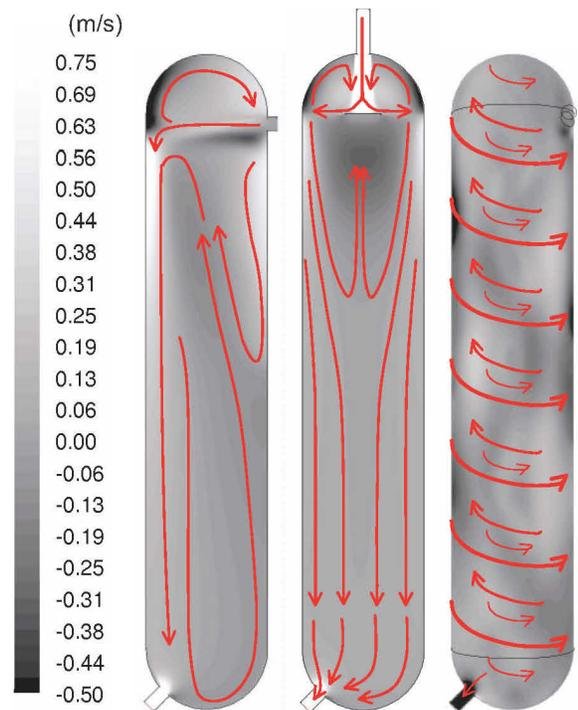
**Figure 4: Comparison of axial velocity and the characteristic flow patterns in the digester with a normal, central, and tangential slurry inlets.**
