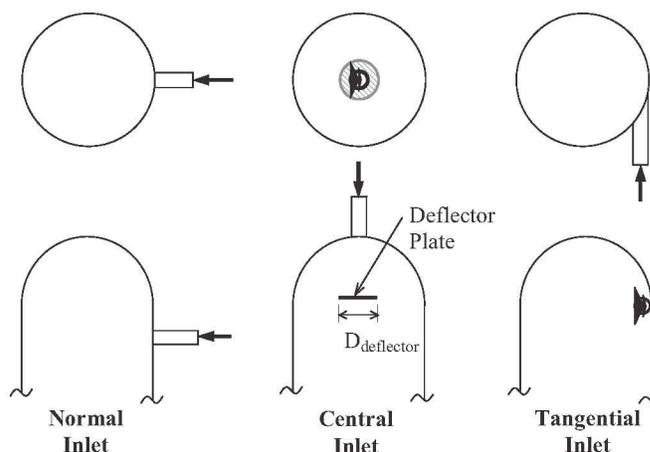
Figure 2: Schematic of the three slurry inlet nozzle configurations considered.
