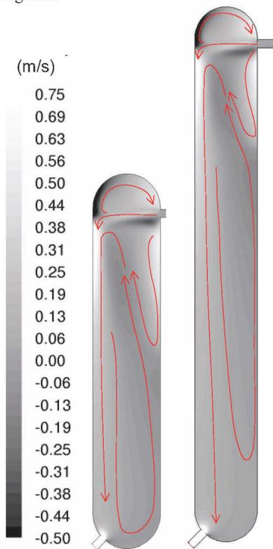
**Figure 3: Comparison of axial velocity and the characteristic flow patterns in the digester for aspect ratios of 4:1 and 7.5:1.**
