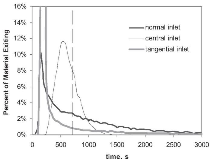
Figure 5: Single digester RTD. Aspect ratio = 4:1.
