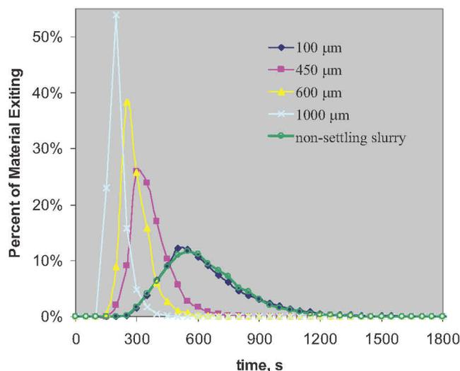
**Figure 7: Solid Particle RTD (central inlet, Aspect ratio = 4:1).**
