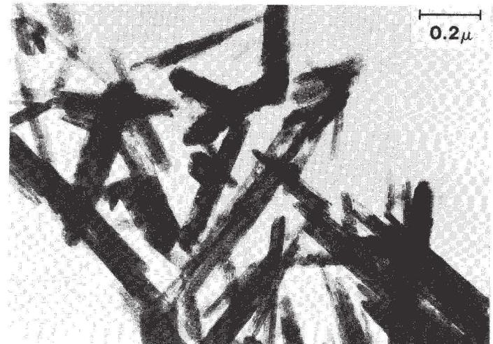
Figure 3 - TEM micrographs of (a) goethite, and (b) goethite calcined at 400°C.
