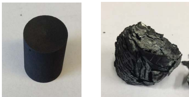
Figure 4. Graphite sample after reaction with sodium vapor [left] and sodium liquid [right].
