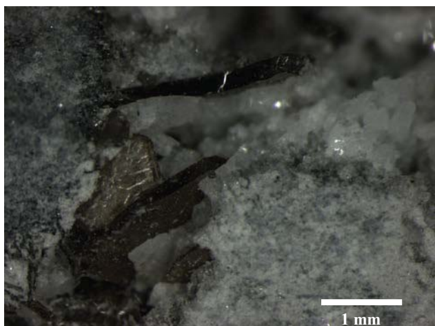
Figure 4. Alumina crystals observed by optical microscope.
