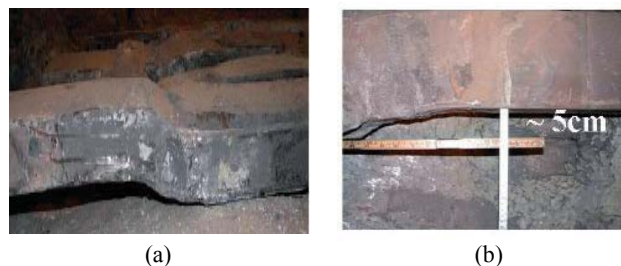
Figure 1: Deformation of the collector bar: (a) deformed collector bar, (b) measurement of deformed collector bar after service life. Extract from [2].
