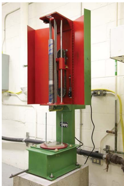
Figure 1. Apparatus used for ramming paste compaction: Proctor Mechanical Rammer
