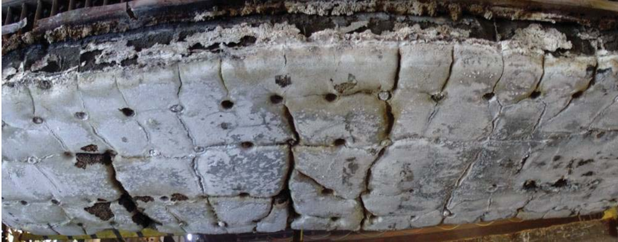
Figure 14: Problematic condition of anode bottom: channels and stud hole cavities
