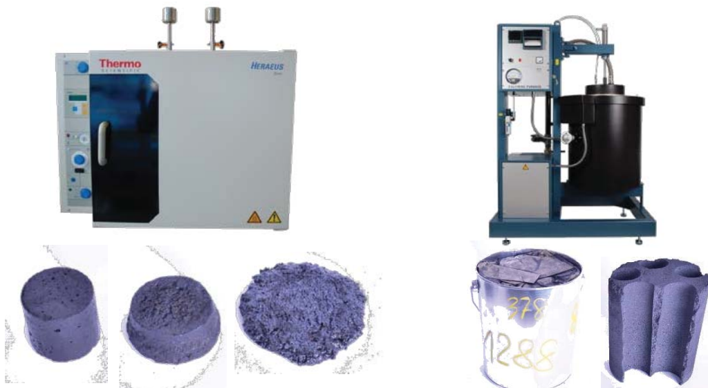
Figure 5: Flowability test on the left, paste baking and core drilled baked anodes on the right
