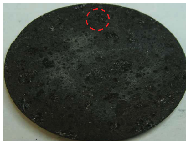
Figure 2. A surface crack formed during baking (visual inspection).
