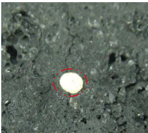
Figure 7. Crack caused by the presence of an impurity
