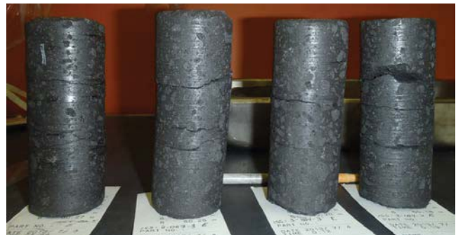
Figure 3 – Batch of green anodes core sample after destructive laboratory tests
