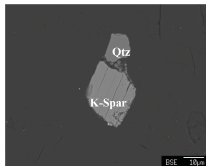
Figure 2: Polished cross-section showing K-feldspar and quartz
