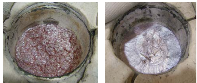
Brand Y Brand X Figure 9. Surface of metal after 5 hour oxidation test.
