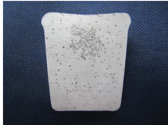
Fig.6 Morphology of samples degassed with absorber solidified under reduced pressure (time = 90s)
