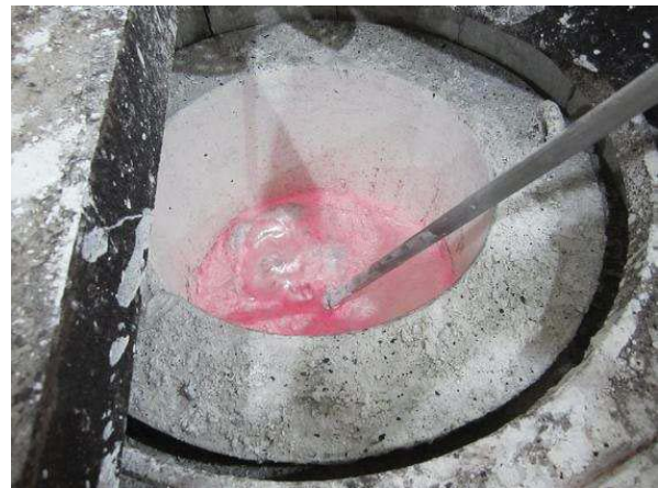
Fig.3 Vacuum degassing with a porous absorber immersed in the melt
