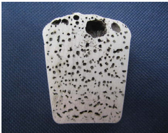
Fig.5 Morphology of samples without degassing solidified under reduced pressure (time = 90s)
