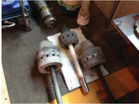
Figure 3. Some of the different rotor materials and designs that were tested.
