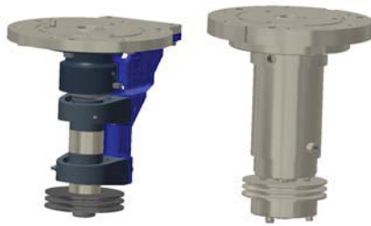
Figure 4. The new rotor bearing package (left) compared to the standard version (right).
