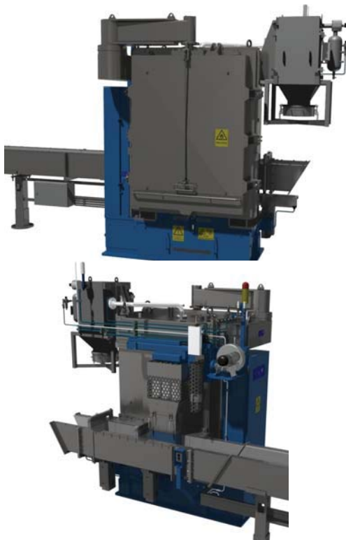
Figure 5. The new dust filter on the I-60 SIR. The filter is placed on top right corner of the top figure.
