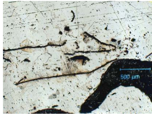
Figure 10: Micrograph from an inlet of a filter. The oxide films are clearly seen and are up to several mm long.
