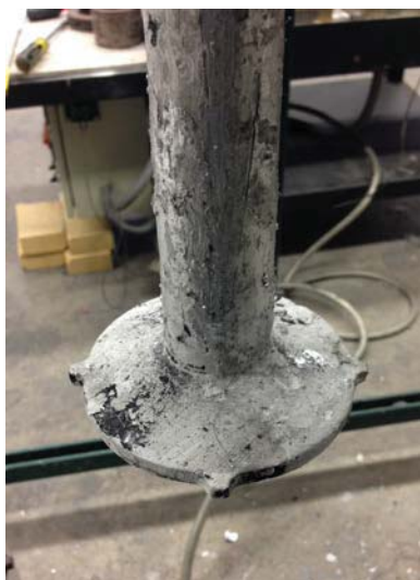
Figure 3: Degasser head after use (Four 1.5 mm outlets, 10.2 cm disk diameter, 3.8 cm shaft diameter).
