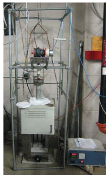
Figure 4: LIBS Probe immersed in the furnace
