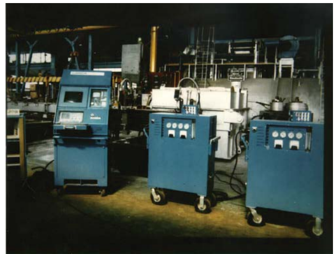
Figure 2: The LiMCA I, the first industrial LiMCA system
