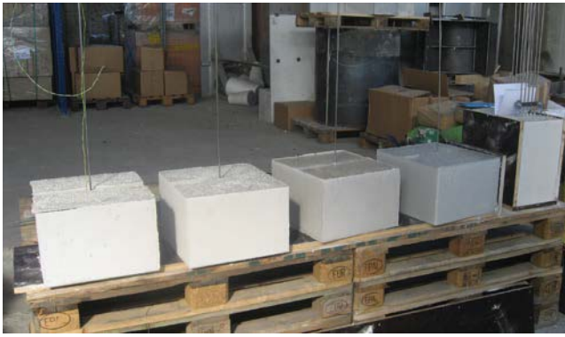
Figure 1: casted monolithic blocks equipped with different sensors
