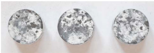
Fig. 19 AlSi30 RS alloy in F condition after the salt spray test (300h) with deposited corrosion products
