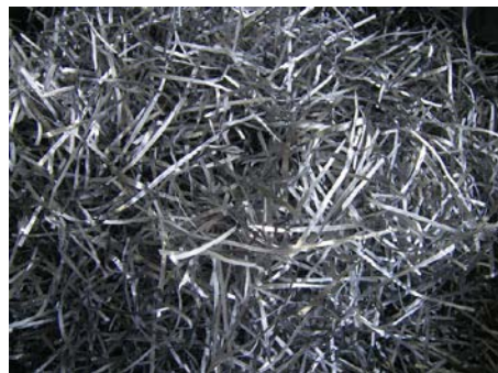
Fig. 1 AlSi30 alloy ribbon cast by RS
