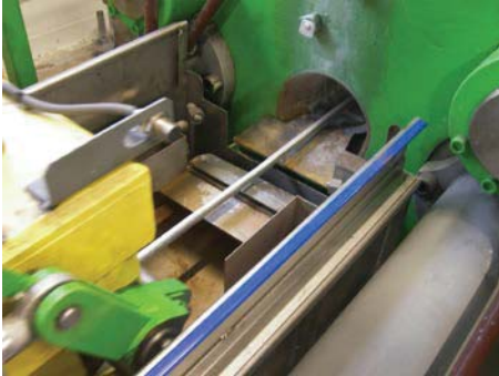
Fig. 3 The process of Ø 18 mm rod extrusion from AlSi30 alloy
