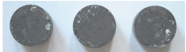
Fig. 21 AlSi30 RS alloy in F condition after the salt spray test (300h) with removed corrosion products
