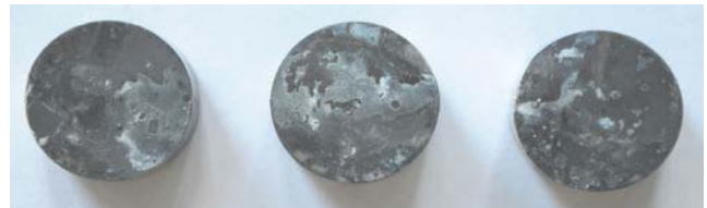
Fig. 22 AlSi30 RS alloy in T6 condition after the salt spray test (300h) with removed corrosion products
