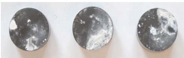
Fig. 20 AlSi30 RS alloy in T6 condition after the salt spray test (300h) with deposited corrosion products
