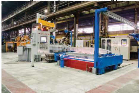
Figure 7. Photograph of R&D casting pit taken from the casting table side.
