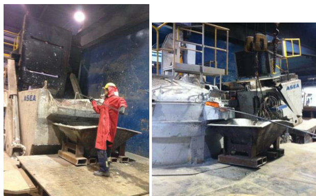
Figure 3 Dross sampling from the melting furnace (left) and the holding furnace at the remelter (right)
