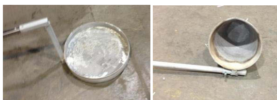
Figure 2 Dross sampling devices: sieve (left) and cup (right)
