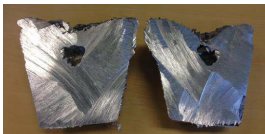
Figure 6 Al dross sample taken with cup from the furnace for charge P2.
