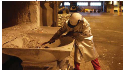
Figure 5 Dross sampling from the dross pan at primary producer
