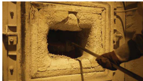
Figure 4 Dross sampling from the furnace at primary producer
