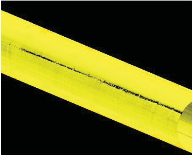
Figure 6 – Example of an inspected defect (vertical tear)
