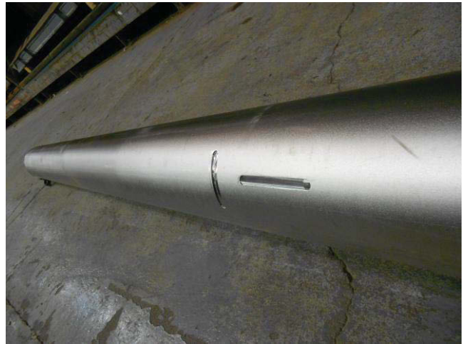
Figure 8 – Control tube with machined reference
