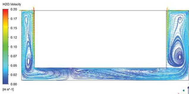
Fig. 16 Water velocity distribution and streamlines at plane LC
