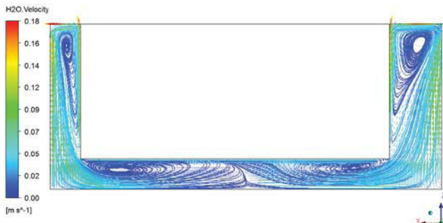
Fig. 15 Water velocity distribution and streamlines at plane LB
