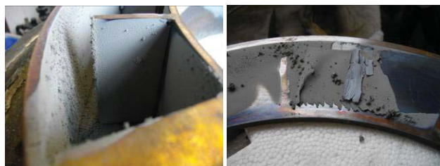
Figure 15: Powdered “metallic” material collected at the copper condenser after the experiment.
