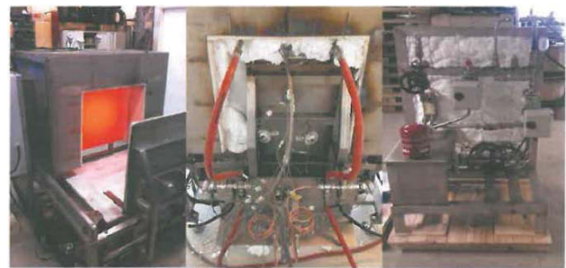
Figure 2. Thermosyphon assembly test setup at the Goodtech laboratory [11]
